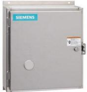
Non-reversing NEMA contactor, Size 4, Three phase full voltage, Contactor amp rating 135A, 3 wire (NO aux included), 220-240/440-480VAC 60Hz coil, Noncombination type, Encl NEMA type 4X 304 S-Steel, Water/dust tight noncorrosive, Extra-wide enclosure
