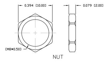
NOTE: MATERIAL HOUSING: PBT UL94V-0, BLACK CONTACT: BRASS SHELL BRASS NUT: BRASS □-RING: EPDM, BLACK FINISH: CONTACT: GOLD PLATED **DVER 50u" NICKEL** SHELL: NICKEL NUT: **NICKEL ELECTRICAL** RATED CURRENT: 1.5A RATED VOLTAGE: 30V INSULATION RESISTANCE: 100 MOhms MIN. 10 mOhms MAX. CONTACT RESISTANCE: IP67 WATER PROOF: **ENVIRONMENT**
