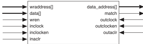
Figure 23. APEX 20KC CAM Block Diagram
