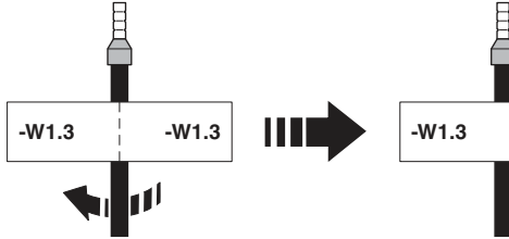
Figure 4-7 Example of a cable flag
