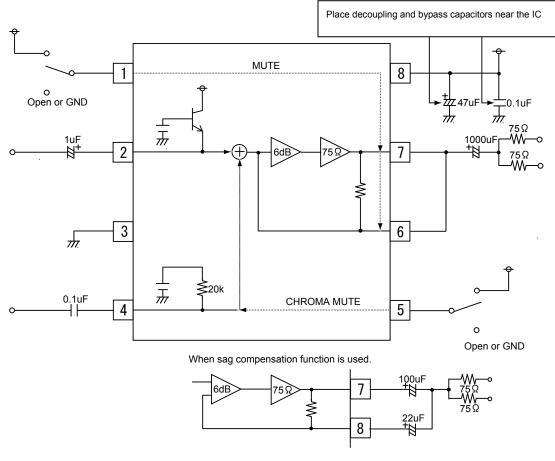
Make sure to take into account the tolerance characteristics of the external components, as well as the IC power dissipation limits.
