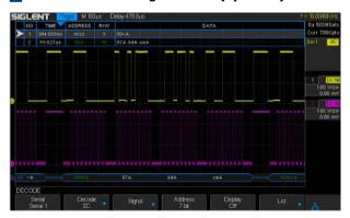
SDS1000X/SDS1000X+ displays the decoding through the events list. Bus protocol information can be quickly and intuitively displayed in table form.
