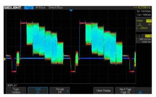
The color temperature display is similar to the intensity-graded trace except that the trace occurrence is represented by different colors (color "temperature") as opposed to changes in the intensity of one color. Red represents the most common occurrences or probabilities while blue is the least common points.
