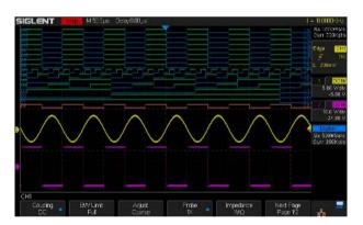
2 analog channels plus 16 digital channels enables users to acquire and trigger on the waveforms then analyze the pattern, simultaneously with one instrument.
