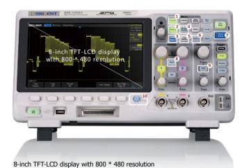
Most commonly used functions are accessible using 10 different one-button operation keys: Auto Setup, Default, Cursor, Measure, Roll, History, Persist, Clear Sweep, Zoom, Print
