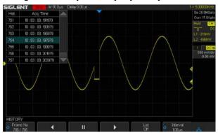
Playback history waveform to observe unusual events and locate the source quickly through the cursor or measurements, located on the keyboard Panel, this function is easily enabled. Segmented memory collection will store the waveform into multiple (up to 80,000) memory segments, each segment will store a triggered waveform and dead time information
