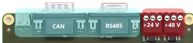
Figure 3: Power; Communication and USB-C connectors of TMCM-BB1
