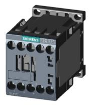
power contactor, AC-3, 12 A, 5.5 kW / 400 V, 4-pole, 42 V AC, 50/60 Hz, main contacts: 2 NO + 2 NC, screw terminal, size: S00
