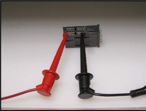
Figure 2- Front to Back IR test setup
