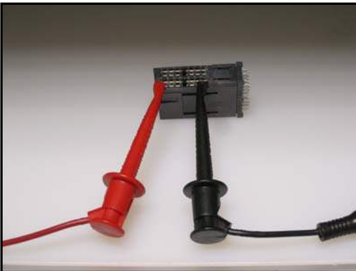
Figure 4- Front to Back Withstand Voltage test setup
