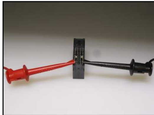
Figure 5- Left to Right Withstand Voltage Test setup
