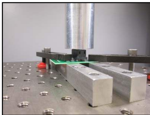
Figure 11- Typical Compliant Pin mounting force onto PCB test setup.
