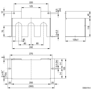
General tolerances according to ISO 2768-cL Dimensions in mm
