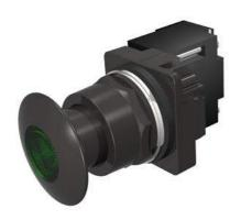
30mm BlackMax, Epoxy Coated Corrosion Resistant Complete Metal Unit Illuminated Push-Pull Operator Transformer type, 600V AC LED Lamp Mushroom Head Cap Small 1 3/4" (44.5 mm) Metal, Black with Green Lens 2 Position Maintained, Pull-to-Release UL Listed, CSA Certified NEMA 1,3,3R,4,4X,12,13 & Automotive Standards
