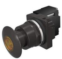
30mm BlackMax, Epoxy Coated Corrosion Resistant Complete Metal Unit Illuminated Push-Pull Operator Transformer type, 600V AC LED Lamp Mushroom Head Cap Small 1 3/4" (44.5 mm) Metal, Black with Amber Lens 2 Position Maintained, Pull-to-Release UL Listed, CSA Certified NEMA 1,3,3R,4,4X,12,13 & Automotive Standards
