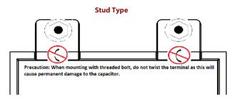
Hardware: M5 =#10 stud / bolt Copper flat washer, #10 or M5 washer with (~.500") OD
