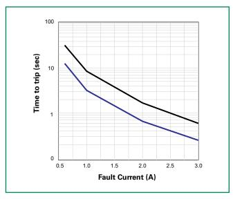
The average time current curves and Temperature Rerating curve performance is affected by a number or variables, and these curves provided as guidance only. Customer must verify the performance in their application.
