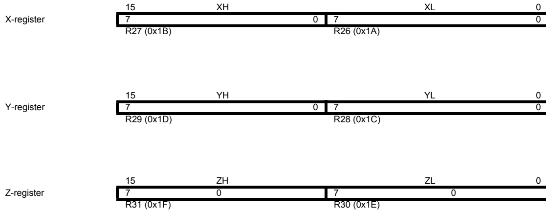
Figure 4-3. The X-, Y-, and Z-registers
