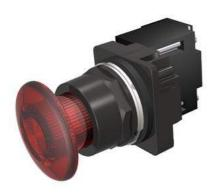
30mm BlackMax, Epoxy Coated Corrosion Resistant Complete Metal Unit Illuminated Push-Pull Operator Full Voltage, 24V AC/DC LED Lamp Mushroom Head Cap Small 1 3/4" (44.5 mm) Plastic, Red 3 Position Momentary UL Listed, CSA Certified NEMA 1,3,3R,4,4X,12,13 & Automotive Standards
