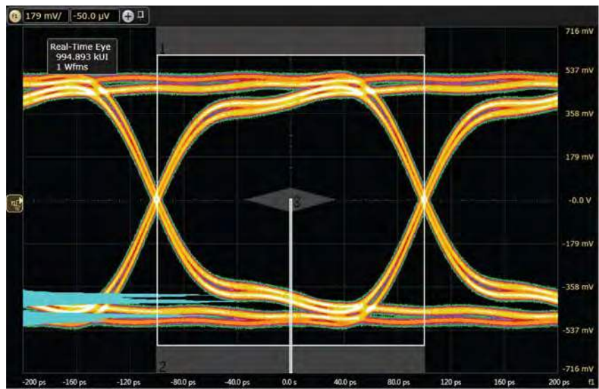
Fig 7. USB 3.1 eye diagram, test board with PCMF2USB30; typical values
