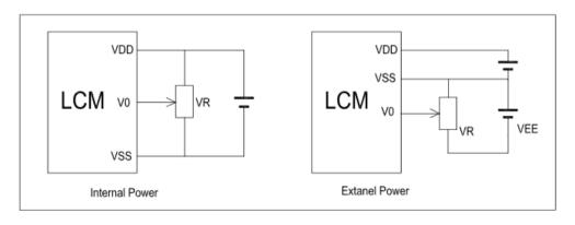
VDD-V0: LCD Driving Voltage
