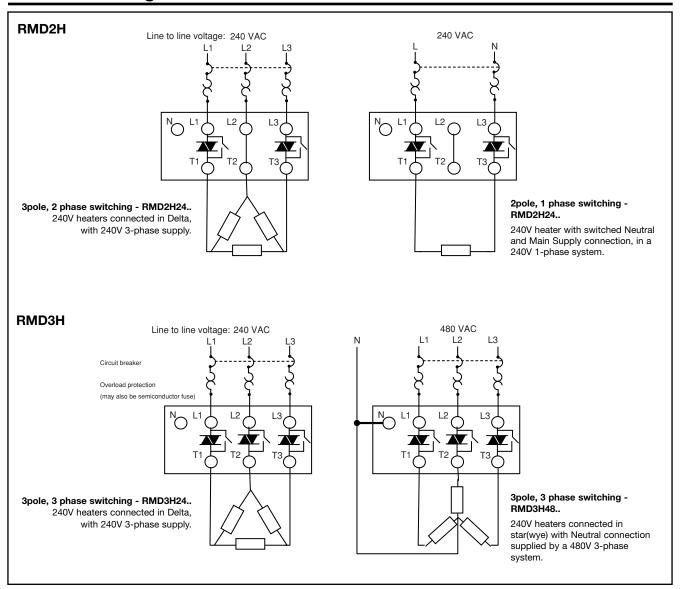
WARNING: Internal power supply in RMD2H and RMD3H24 is taken through terminals L1-L3, while for RMD3H48 it is taken through L1-N. If these are not connected correctly, the internal bypass relays will not work. The 'N' terminal must be left unconnected for RMD2H and RMD3H24.
