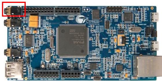
Figure 2-21. I2S Headphone Test
