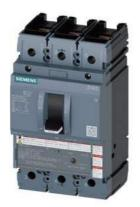
circuit breaker 3VA5 UL frame 250 breaking capacity class C 100kA @ 480 V 3-pole, line protection TM230, FTAM, In=175A overload protection Ir=175A fixed short-circuit protection Ii=5...10 x In UL489 SB (naval), 50 deg. cel. nut keeper kit on both sides
