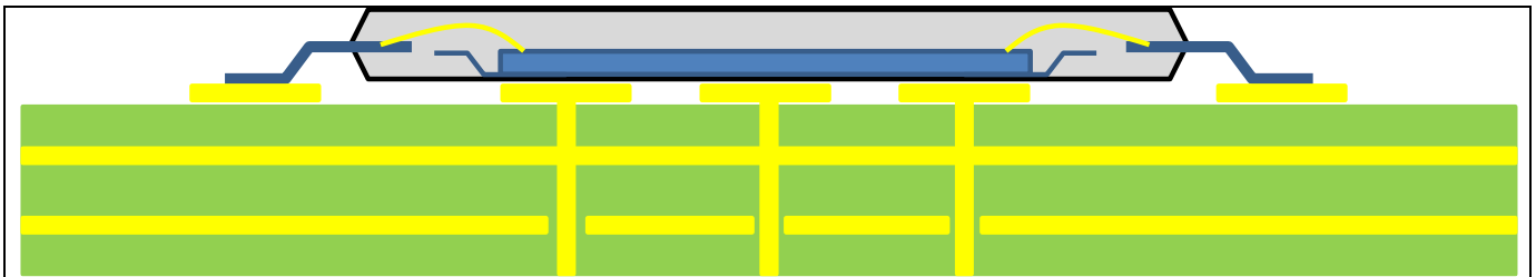
Figure 7-1: Example Thermal Via Holes on PCB.
