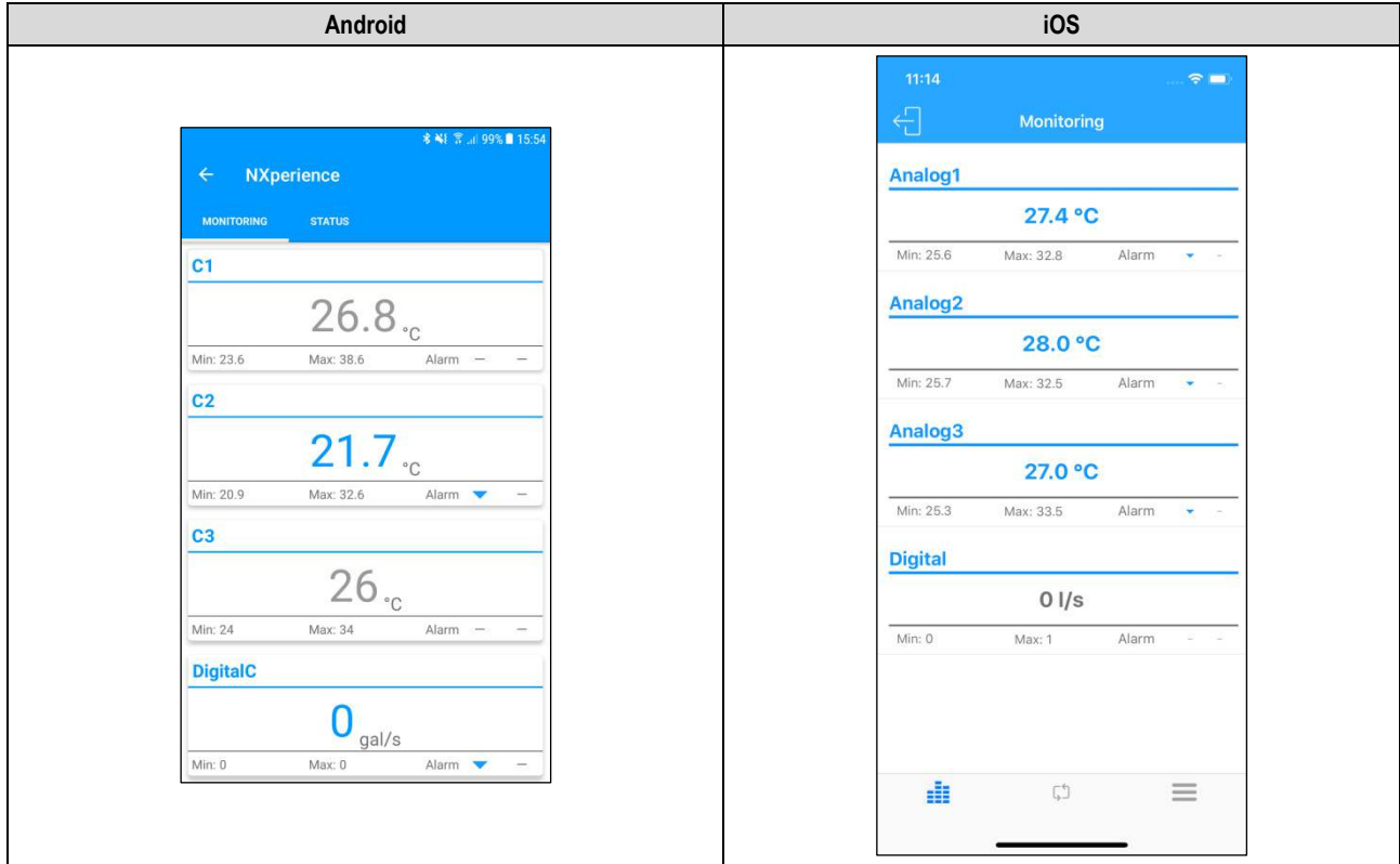
Figure 34 – Monitoring: Low Alarm
