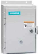
Non-reversing motor starter, Size 1, Three phase full voltage, Solid-state overload relay, OLRelay amp range 3-12a, 24VAC 50-60HZ coil, Non-combination type, Enclosure type 12, Dust/drip proof for indoors, Extra-wide enclosure
