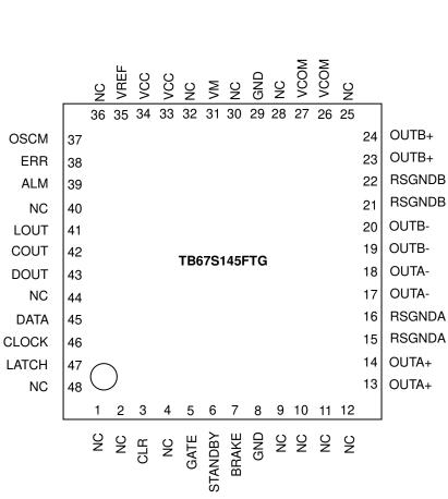
(\*) Please mount the four corner pins of the QFN package and the exposed pad to the GND area of the PCB.
