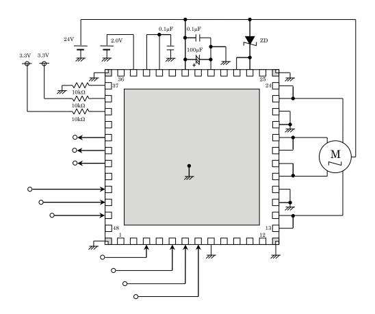
Please mount the four corner pins of the QFN package and the exposed pad to the GND area of the PCB.
