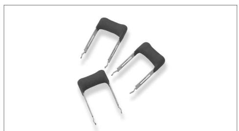
The resistive element comprises a metal oxide film deposited on a ceramic former. The element is protected by a flameproof coating which will withstand overload conditions without flame or mechanical damage. They are recommended for use in applications such as line protection, automotive. TV's, switch mode power supplies, etc...
