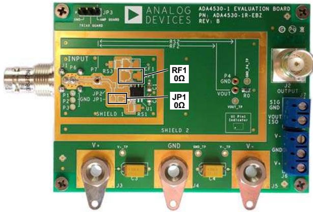
Figure 5. Buffer with Triax Guard Externally Driven
