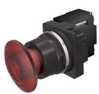
30mm BlackMax, Epoxy Coated Corrosion Resistant Metal Operator, Round Illuminated Twist-to-Release Transformer type, 240V AC Incandescent Lamp Mushroom Head Cap Small 1.79" (45 mm) Plastic Cap, Red 2 Position Maintained, Twist-to-Release UL Listed, CSA Certified NEMA 1,3,3R,4,4X,12,13 & Automotive Standards
