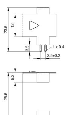
Dimensional tolerances +/-0,2 Dimensions in mm
