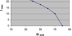
M ax. allo wable ambient Temp. at specific current (rms) B25667C6137A375
