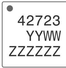
Figure 19 • Package Marking Specifications for PE42723
