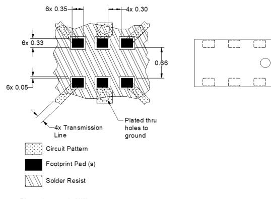
Dimensions are in Millimeters Mounting Footprint
