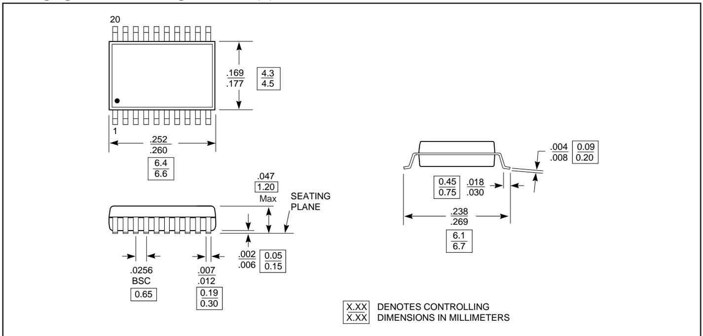
**Packaging Mechanical: 20-pin SSOP (H)**
