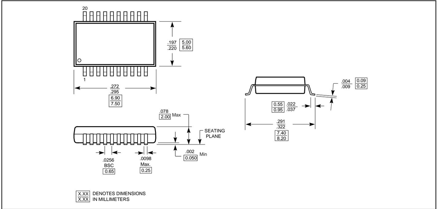
**Packaging Mechanical: 20-pin SOIC (S)**
