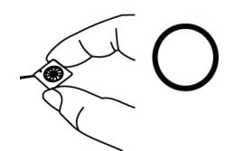
Don't pull fan with lead wires.
