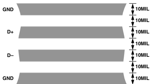
Figure 8. Arrangement of Signal Tracks
