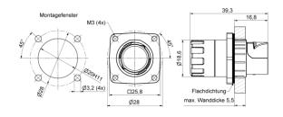
Main Dimensions Extension \*for max. wire cross-section pay attention to the cross-section of used contacts
