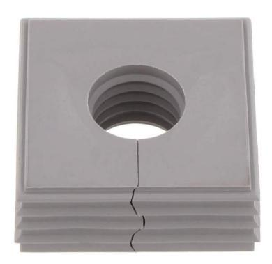
Seal, Mounting type: Plug in, Length x width: 42.8 mm, Max. cable diameter: 18 mm, IP 66, Colour: Grey
