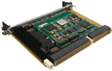
Figure 3: Curtiss Wright VPX6-187 based on the QorIQ P4080 processor
