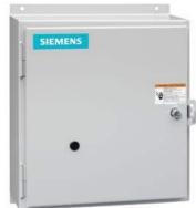
Mechanically held lighting contactor, Contactor amp rating 60Amp 0NC  $\_$  6NO poles, 550VAC 50HZ/600VAC 60HZ coil, Non-combination type, Enclosure NEMA type 1, Indoor general purpose use
