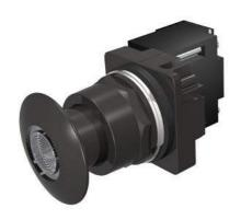
30mm BlackMax, Epoxy Coated Corrosion Resistant Complete Metal Unit Illuminated Push-Pull Operator Transformer type, 480V AC LED Lamp Mushroom Head Cap Small 1 3/4" (44.5 mm) Metal, Black with Clear Lens 3 Position Momentary UL Listed, CSA Certified NEMA 1,3,3R,4,4X,12,13 & Automotive Standards
