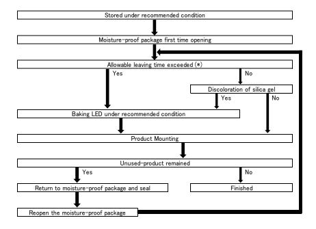
Allowable leaving time means the maximum allowable leaving time after opening package, which depends on each LED type.
