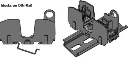
Place one edge of DIN-Rail in fuse block base, then rotate block down until it clicks into place.
