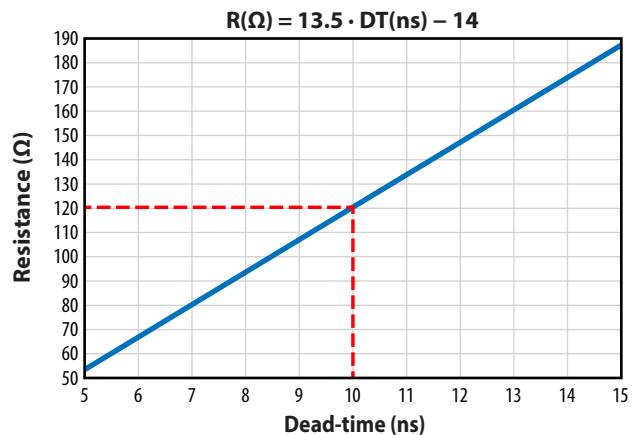
Figure 4: The required resistance values for R620 or R625 as a function of desired dead-time
