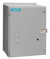
Mechanically held lighting contactor, Contactor amp rating 200Amp 0NC  $\_$  3NO poles, 110VAC 50HZ/120VAC 60HZ coil, Non-combination type, Encl NEMA type 4X 304 S-steel Water/dust tight noncorrosive
