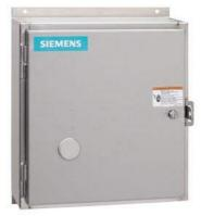
Non-reversing NEMA contactor, Size 2, Three phase full voltage, Contactor amp rating 45A, 3 wire (NO aux included), 24VAC 50-60Hz coil, Non-combination type, Encl NEMA type 4X 304 S-Steel, Water/dust tight noncorrosive, Extra-wide enclosure
