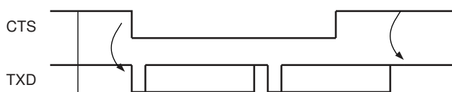
Figure 38-28. Transmitter Behavior when Operating with Hardware Handshaking
