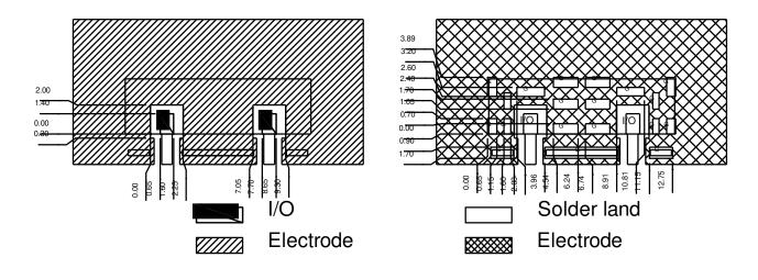
The recommended shielding case layout guide (min)
