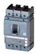
circuit breaker 3VA5 UL frame 250 breaking capacity class H 65kA @ 480 V 3-pole, line protection TM230, FTAM, In=110A overload protection Ir=110A fixed short-circuit protection Ii=5...10 x In cable connection on both sides
