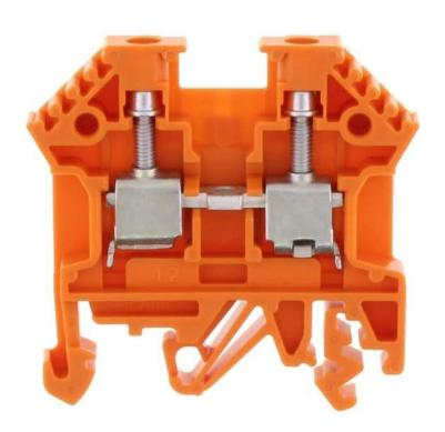
Feed-through terminal, Screw connection, Mounting type: Mounting rail TS 35/7.5 and TS 32, Rated cross-section: 4 mm², Width: 6 mm, Colour: Orange
