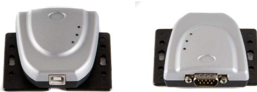
Figure 2.1 – USB2-F-7x01 with UniClip Brackets
